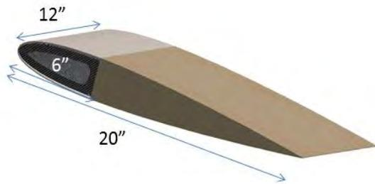
Figure 2a. Basic Design Dimensions
