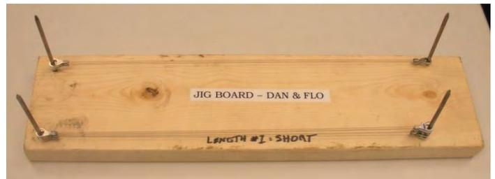
A-3. Jig board used for constructing wires
