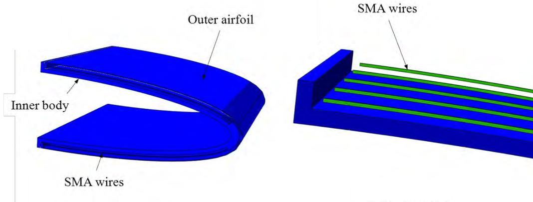
**Figure 3. 3-D Beam Element SMA Approximation Simulation**
