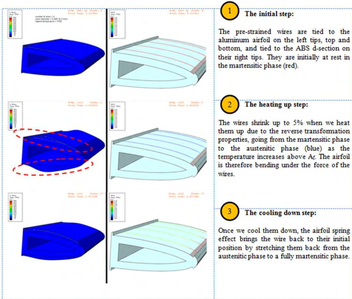
A-1. Transformation Path of SMA Wires in Software Analysis
