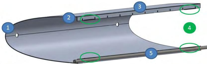
Figure 7. Aluminum sheet CAD model
