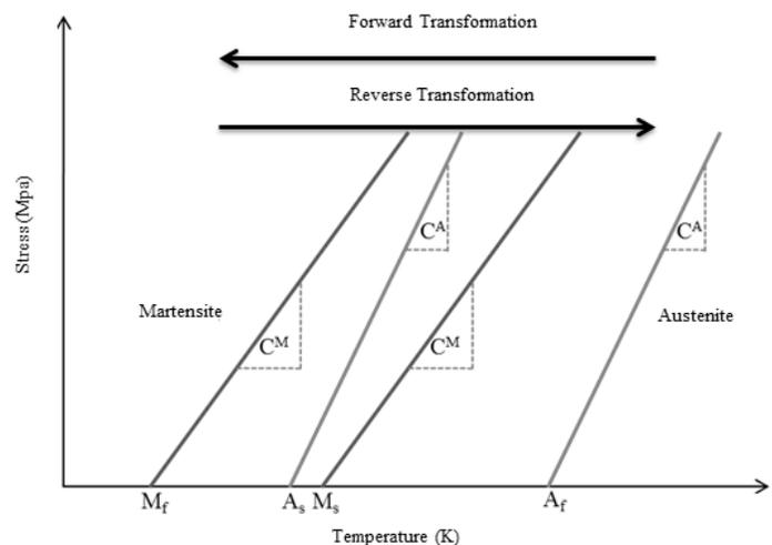
**Figure 1. SMA stress vs. transformation temperature plot**
