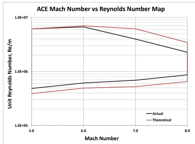
**Fig. 4: Mach Number vs Reynolds number. The black line indicates the current operational limits while the red line is the theoretical limit if the air in the settling chamber was 533 K [2]**
