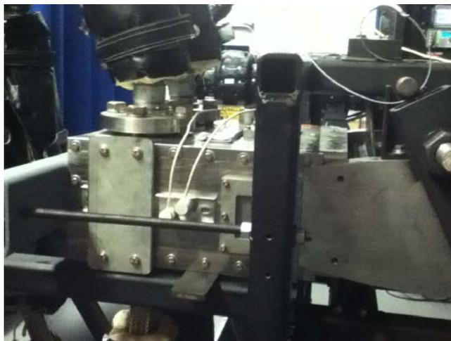
**Fig. 6: Settling chamber with strip heaters installed and wired**
