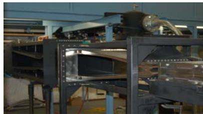
Fig. 1: Side view of ACE tunnel settling chamber, nozzle, expansion chamber, and diffuser
