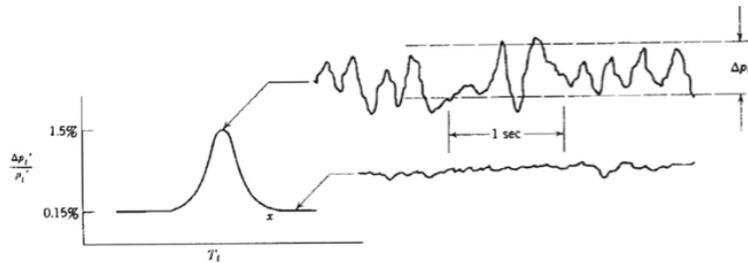
Fig. 2: Fluctuations in Pitot pressure readings in the presence of liquefaction[1]
