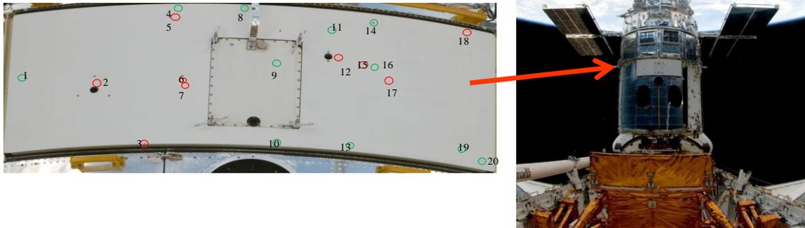
Figure 7. 20 largest impact features seen on the Hubble WFPC2 camera radiator. The red circles are features identified during a 2002 repair mission. Impact features in green circles were created between 2002 and 2009.
