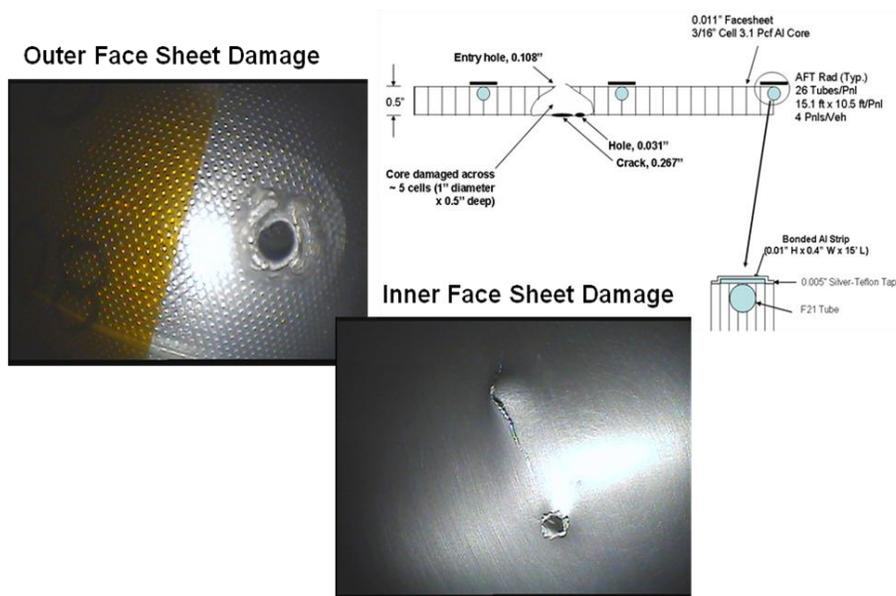
Figure 5. – Impact feature seen on STS-115 radiator. The entry hole is 2.7 mm diameter which created a 2.5 cm void in the radiator’s honeycomb structure.
